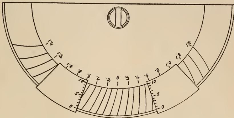
FIG. 3.—Diagram to show the design of an apertometer with a diagonal scale, thus giving direct readings to 0.01 N.A.
